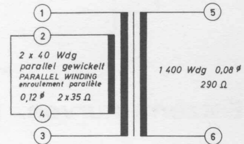
BV 9030—527 Treibertrafo DRIVER TRANSFORMER Transfo driver
